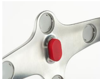
Illustration of the positioning of reflective marker in the housings provided on the frontal tracker.
